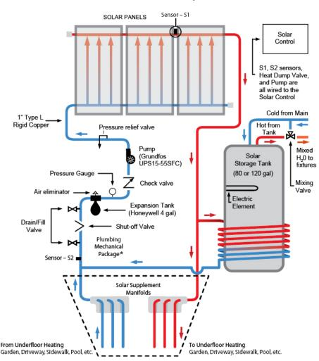
\* Plumbing Mechanical Package includes: Drain & fill valves, shut-off valve, pressure relief valve, pressure gauge, check valve, expansion tank & air eliminator.
