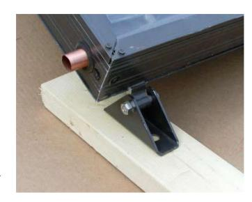
3. If an angle adjustment is not necessary, the rear mounting is the same as for the front. If an angle adjustment is required, the rear AE-Clips are attached to the rear "Triangle Roof Mounting Brackets" via the "Tilt Mounting Struts", using a 3/8" x 1-3/4" SS bolt at the bottom and a 3/8" x 4" SS bolt at the top of each strut.
