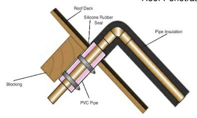
The roof can be penetrated with this detail or with a boot. Seal with silicone sealant, top and bottom and sides.
