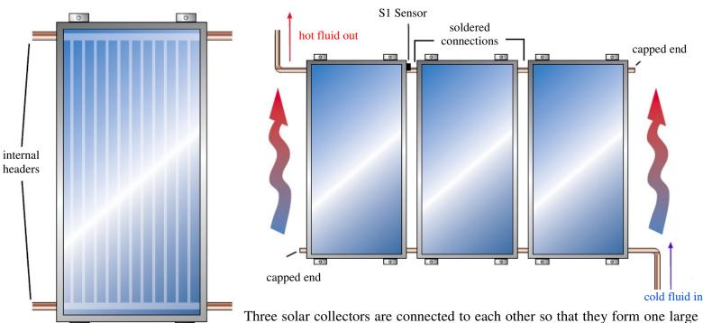
Three solar collectors are connected to each other so that they form one large solar collector array. The collectors have "internal headers" which go across the top and bottom and have outlets on the sides. When the collectors are connected, the headers of each solar collector are soldered to the headers of the others.
