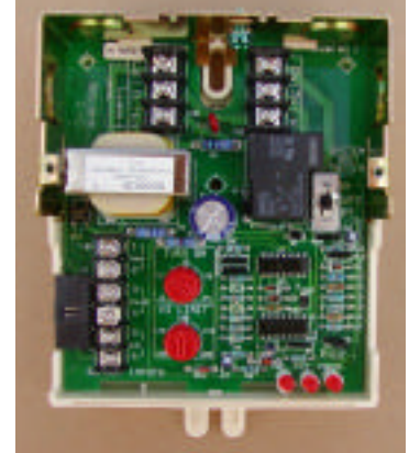
Solar Control (cover off)
