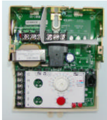
Setpoint Control (cover off)
