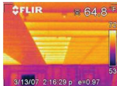
It is seen that ordinary paper is nearly useless in retarding back losses whereas the reflective barrier is effective in reflecting much of the heat that would otherwise be lost. In the thermograph (above right), the material covering the floor joist on the left is aluminum foil backed paper. Its temperature is 64 degrees F. The shorter length of material on the right is ordinary paper without a foil facing. Its temperature is 68 degrees F. This is a considerable difference.
